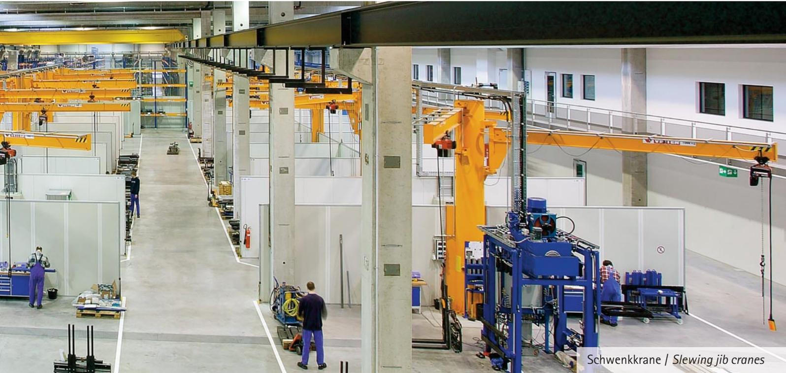
Schwenkkrane / Slewing jib cranes
